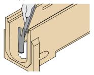
3. A pipe may be fitted into the hole using an appropriate sealant or adhesive.
