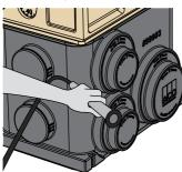
2. Insert pipe into hole and seal using appropriate sealant or adhesive.
