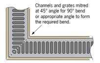
Corners are formed using a mitred joint by cutting channels and grates to the required angle and joining together.
