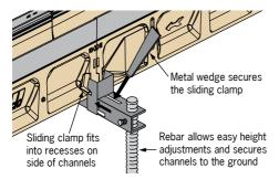
NOTE: Designed for KlassikDrain, PowerDrain and TraffikDrain channels only.
