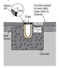
Asphalt can be finished directly up to the channel edge.
