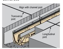
Transverse expansion joints (perpendicular to the channel) may be required to allow movement and prevent surface cracking in the slab.
