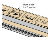
To form a T-junction at a location along a channel that does not have a moulded guide, place another channel perpendicular at the proposed joint location.
