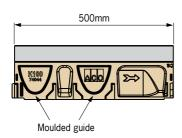
For T-junctions, all half metre channels provide a moulded guide to aid connection.
