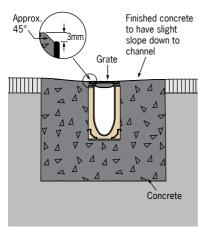
To finish installation, trowel concrete flat and taper down to channel edge. The top of adjacent pavement must be above the grate level (approx. 3mm), this ensures all liquids drain into the channel and protects the edge rail from damage by direct vehicular traffic.
