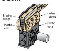
In-line pits have the same width as the channel but deeper. Allows use of rubbish basket to collect debris.
