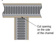
T-junctions or right angle joints are formed when an opening is cut into the side of one channel and another channel is butted up square to this opening.
