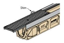
Shims such as washers are to be placed along one side of the grate to maintain the clearance gap that exists before the pour.
