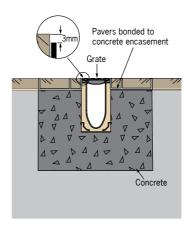
Brick pavers can be installed up to the channel edge.
