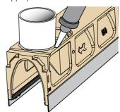
CAUTION: Use a hammer on the knockout symbol ONLY, as damage may occur requiring replacement. Alternative acceptable methods are core drilling or stitch drilling.
