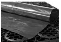
Impermeable geomembranes are for retention and detention applications. For 'non sensitive' applications taped joints are usually acceptable. ACO recommends installation by professional lining contractors for environmentally sensitive applications to acheive a geomembrane system with 100% watertight welded joints.
