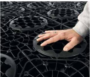
To ensure the geomembrane or geotextile can be wrapped around the tank snugly, covers should only be inserted in the top layer of the ACO StormBrixx<sup>®</sup> system. They prevent the geomembrane or geotextile being forced into the necks of the pillars during backfilling.
