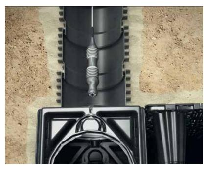
Inspection cameras are introduced into the system through the access shaft.
