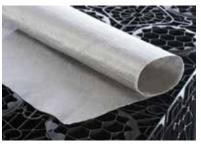
Permeable geotextiles are for use in infiltration applications. They permit the passage of water into and out of the ACO StormBrixx<sup>®</sup> system. Geotextiles are also used to protect the geomembrane from mechanical damage due to ground and thermal movement. They are placed on the outer side of geomembrane.
